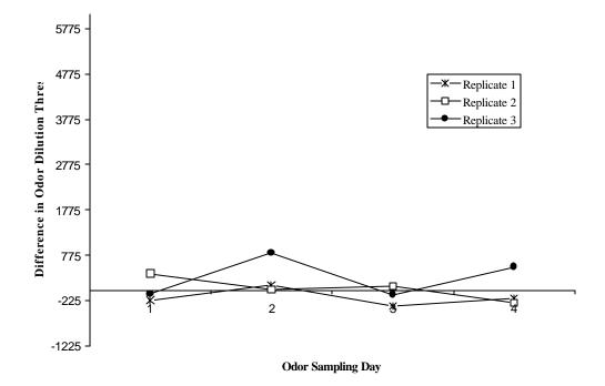
Differences in Hydrogen Sulfide between  $M_2$  Acid Buffer &  $M_2$  Microbial Activator and Untreated Columns by Replicate
